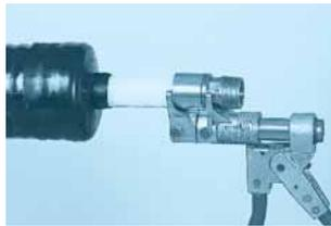
6. With levering movements, push the slider sleeve as far as the collar of the fitting.
