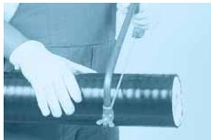
2. Cut the jacket with a pipe-cutter or a saw at the marked distance from the end of the pipe.
