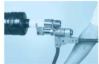
8. Press the levers together again, then swivel the movable lever upwards by 90° to move the tool into its initial position.
