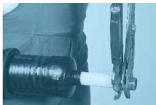
6. Retighten the fitting. Caution: Do not overtighten!
