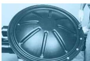
6. Screw the shaft together with the cover, including the sealing ring (screws, washers and nuts are supplied).
