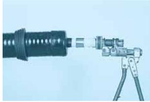
2. Widen the pipe twice, with a 30° offset; the sliding sleeve must not be located in the widened zone.
