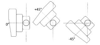
Horizontal Mounting position: The sensor head **MUST** be placed to the side **+/- 45°** in relation to the pipe axis to avoid influences of air inclusions (top) or dirt (bottom).
