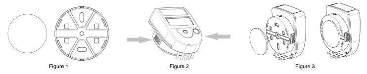
To remove the integrator from the wall support, it will be sufficient to press laterally on the two locking buttons while pulling the assembly towards you. Rewind the connection cable at the position provided for this purpose on the flow meter (1) and re-insert the integrator (2).
